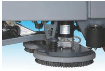
Brush release by foot. No tools required.
