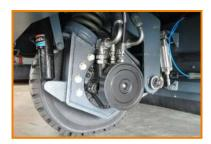
Hydraulically controlled drive wheels designed with powerful shock absorber and suspensions.
