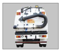
Regenerative Type, truck Mounted Sweeper with capacity of 6 cubic metres and above.
