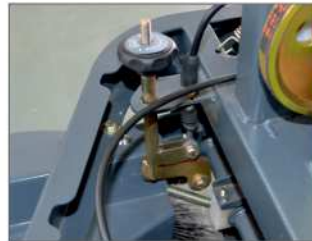
Easy access to broom adjustment system
