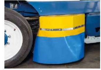
Side brush dust suppression skirts for dry dust-free sweeping.
