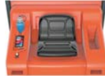
Ergonomic cabin of a decent workplace(air fan, USB charging connector, bottle holders and various storage compartments)
